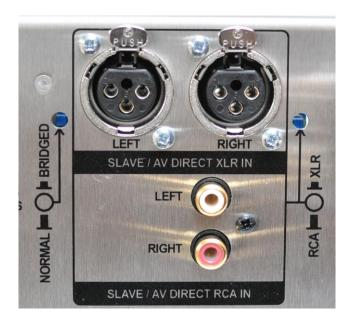
Selecting Bridged mode turns the Hydra II in to a high powered monoblock amplifier, capable of very high output. If using a system consisting of both bridged and unbridged amplifiers, the centre LIPS switch should be set to mono to reduce the gain by 6db which equalises the volume structure across the system. Loudspeakers with a minimum impedance of less than four ohms must not be used with a bridged Hydra II.
